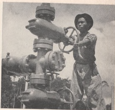
A "CHRISTMAS TREE" in far Sumatra is not as rare as it may seem. To oilmen, it means the assembly of valves and fittings (above) that controls the flow of an oil well.
