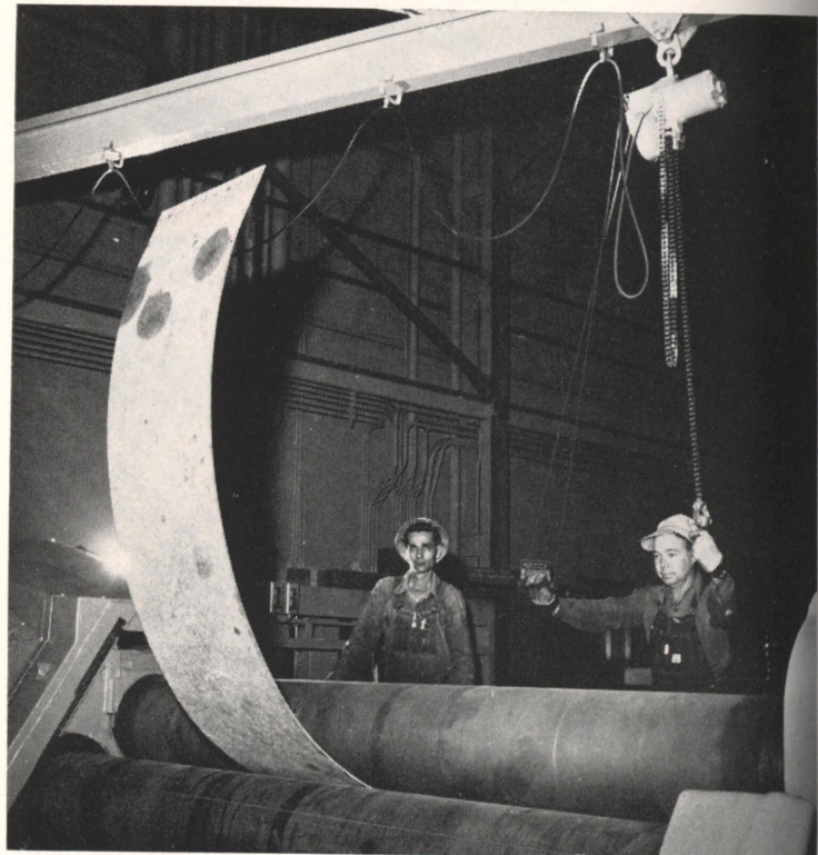
W. I. Peppers, left, operates this plate roll machine while C. T. Burns assists with the hoist. This Boiler Shop machine rolls plate 3/4" thick and 8' long.
