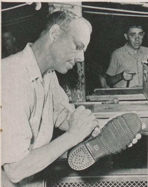
Concrete results of the synthetic rubber program are synthetic rubber boots like these. They're 100% Buna S, except for rubber cement, and are being rationed for essential war and industrial work.
