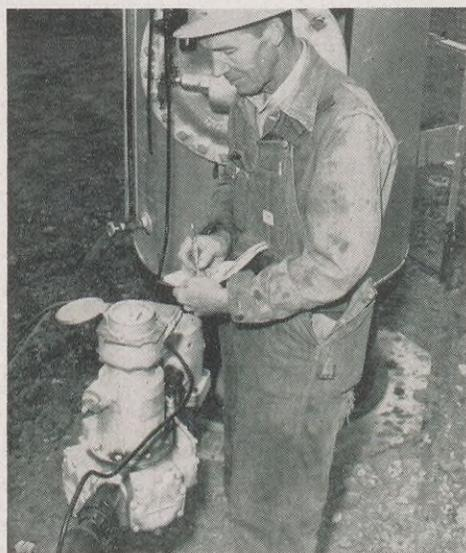
Left, Pumper Wilkins reads a meter which registers quantity of crude oil coming from one of the Big Mineral field producing zones. Below, close to the shore on a fill, a Shell rig drills one of 71 Company-operated wells at Big Mineral.
