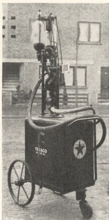
Wheel Tank with Visible Measuring Pump
