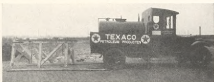
Combination Truck with Sliding Rack for Delivering Drums and Tins
