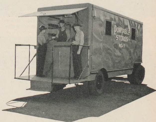
▲ A Portable Store has been placed in service at Wood River to speed materials to the various units spread throughout the huge refinery. The Portable Store is equipped with a telephone so that it can be contacted immediately to answer rush calls.
