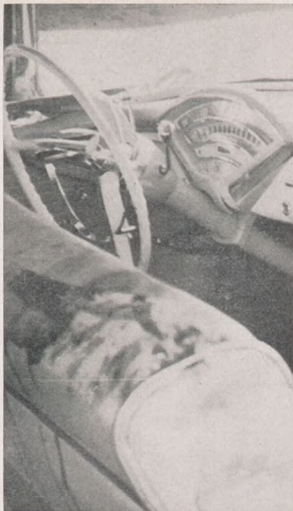
The force-absorbent steering wheel on this car saved the driver from possible fatal injuries in a crash by yielding under impact.
