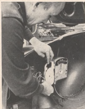
Special speedometer in trunk compartment (left) gave accurate speed record of cars. Fuels (right) were alternated to determine each car's specific octane requirement.
