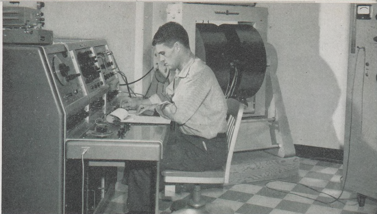
Research Chemist W. E. Putnam operates the latest tool for chemical analysis, the nuclear magnetic resonance spectrometer, located in the Physics Laboratory.
