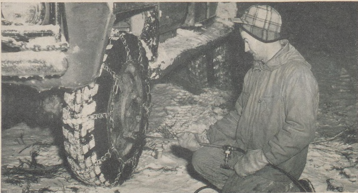
1. Seismic Helper K. T. Reese of the Calgary Area's Seismic Party 192 starts his morning by using a blow torch to thaw the wheels of a recording unit truck frozen during the 50-below-zero night. The tire chains are essential for driving through snow-covered terrain.
