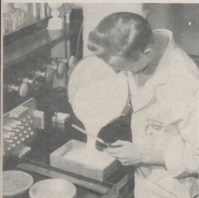
Preparing for the last step in making a sample of foam rubber, Laboratory Assistant E. E. Ewins pours whipped liquid latex into the mold in which it will be cured.
