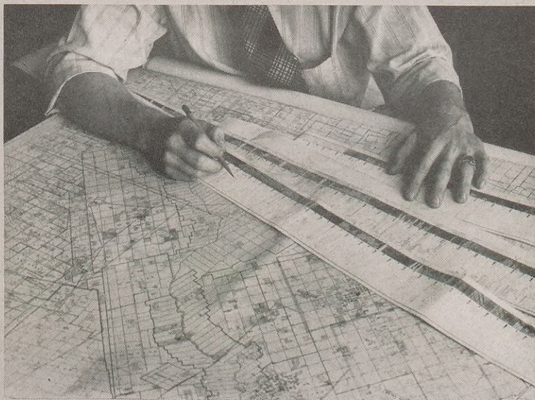
From data furnished by field parties, map makers project contour lines on maps so hidden structure of underground formations may be interpreted.
