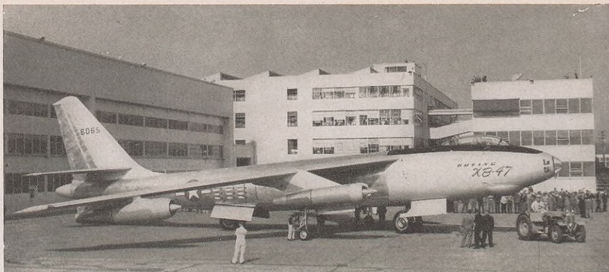
The Army experimental jet bomber XB-47 has a radical design and is propelled by six turbo-jet engines, three fixed to each wing.
