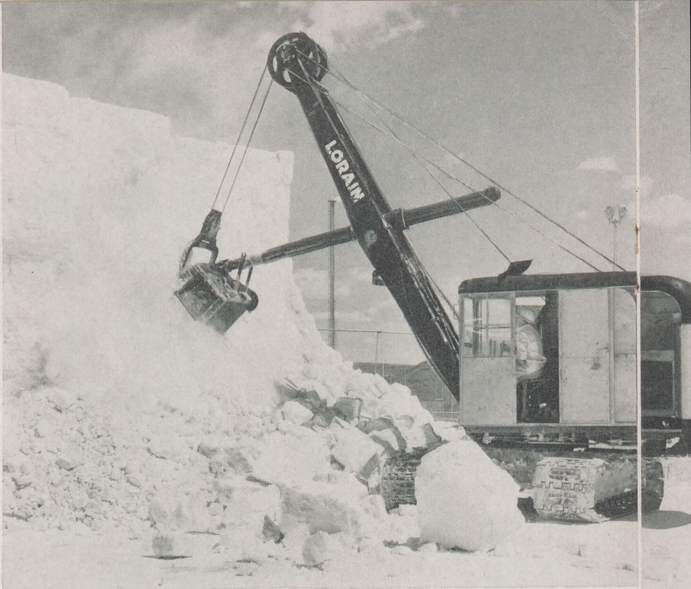
A steam shovel chews into a hill of sulfur at Shell's Jumping Pound plant in Alberta, Canada. Jumping Pound produces about 30,000 tons of sulfur per year.
