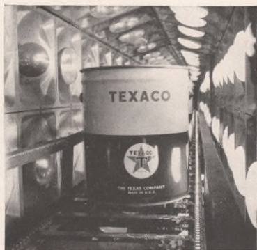
Texaco makes most of its own containers. Paint on pails is dried by infrared heat.
