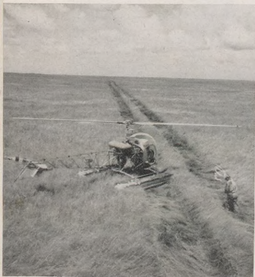
In some locations, seismic crews use both helicopters and marsh buggies. The aircraft (left) setting down near a marsh buggy track is used by men who set out and recover seismometers. The cumbersome marsh buggy (center) tows shooting and recording equipment to the proper locations in the marshes. At right, crew members stand by the seismic recording instrument as they await the detonation of an explosive charge.
