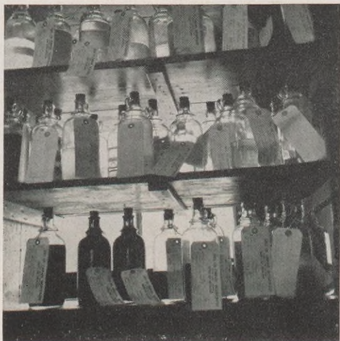
Tested samples are kept on hand for 24 hours for spot rechecks. Sometimes specially blended lube oils are retained as long as six months for this purpose.
