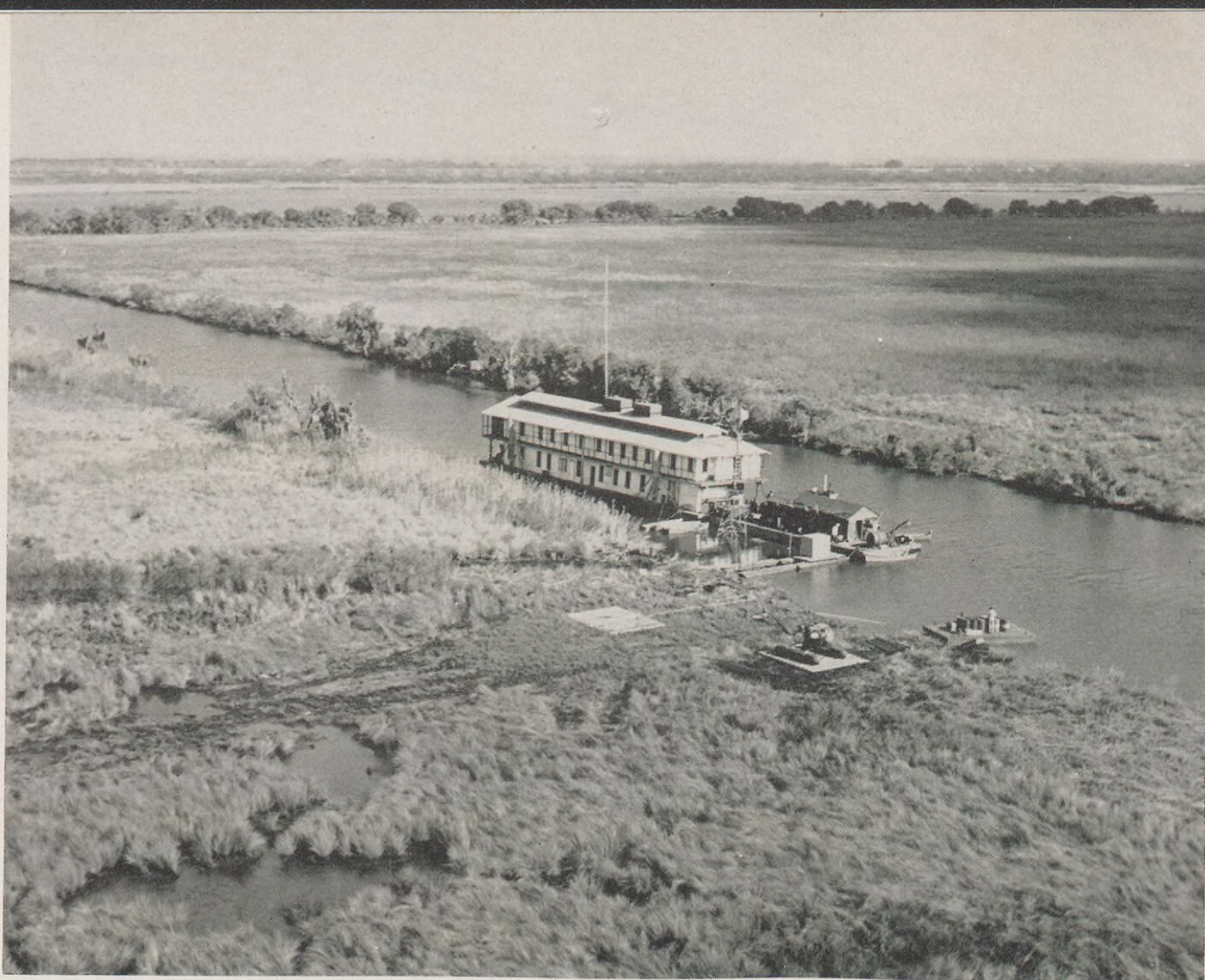
Crews carrying out seismic operations in the Louisiana marshlands work out of a base camp such as the one illustrated in the picture above. This temporary outpost is made up of a "quarter boat" anchored in the bayou—in which the men eat and sleep—loading strips for the helicopters, and auxiliary work barges and launches. The men are taken to and from their working locations in the marsh each day by helicopter.
